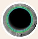
Cross-section of one hollow fiber membrane
